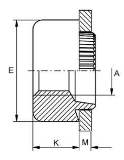
Female thread A = M2,5Height K = 3.0Outer diameter E = 8.0Plate thickness = 4.1 to 4.3
